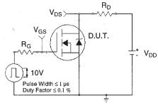
Fig 10a. Switching Time Test Circuit
