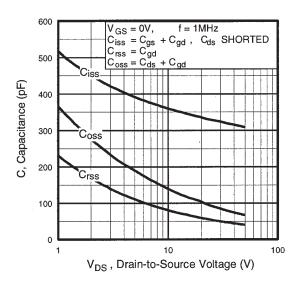
**Fig 5.** Typical Capacitance Vs. Drain-to-Source Voltage
