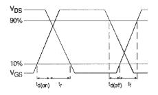
Fig 10b. Switching Time Waveforms
