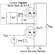
Fig 9b. Gate Charge Test Circuit
