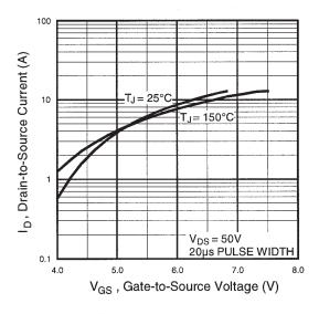
Fig 3. Typical Transfer Characteristics
