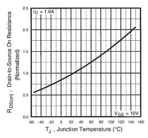
**Fig 4.** Normalized On-Resistance Vs. Temperature
