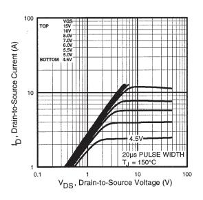
Fig 2. Typical Output Characteristics,
