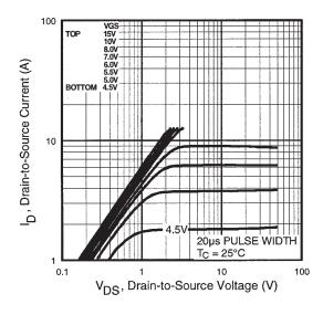
Fig 1. Typical Output Characteristics,
